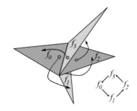
VF relation does not involve any dynamic allocation, the chain of face is distributed onto the involved face
