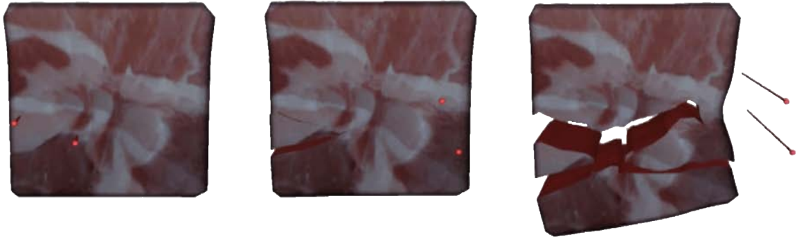
Figure 2.11: Example of cut with multiple advancing fronts using the Splitting Cubes, frames captured during an interactive simulation. The cut path is defined by the counter clock-wise motion of the two blades.
