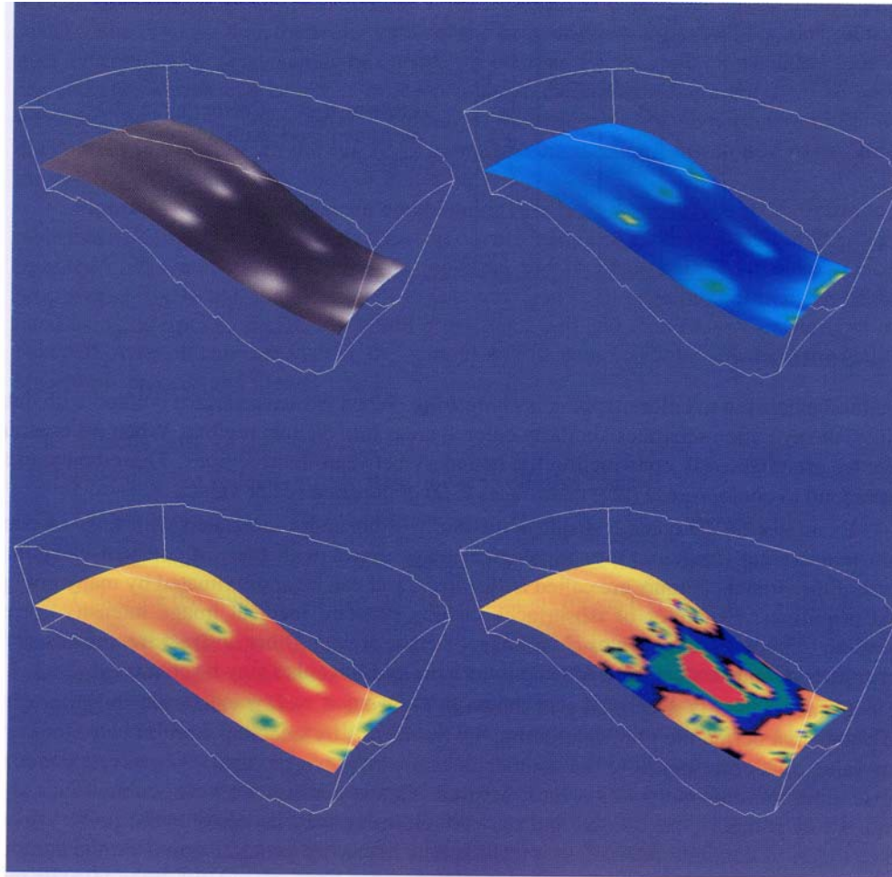
Figure 6-3 Flow density colored with different lookup tables. Top-left: grayscale; Top-right rainbow (blue to red); lower-left rainbow (red to blue); lower-right large contrast ( rainbow.tcl ).
