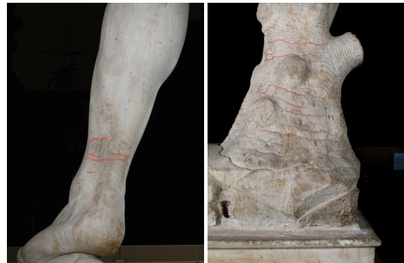
Figure 1: The two images show the regions affected by the fractures (the back of the left leg and the so-called "broncone", i.e. the tree stump on the back of the right leg), most of them extremely thin. Images courtesy of A. Borri (BORRI et al, 2004).
