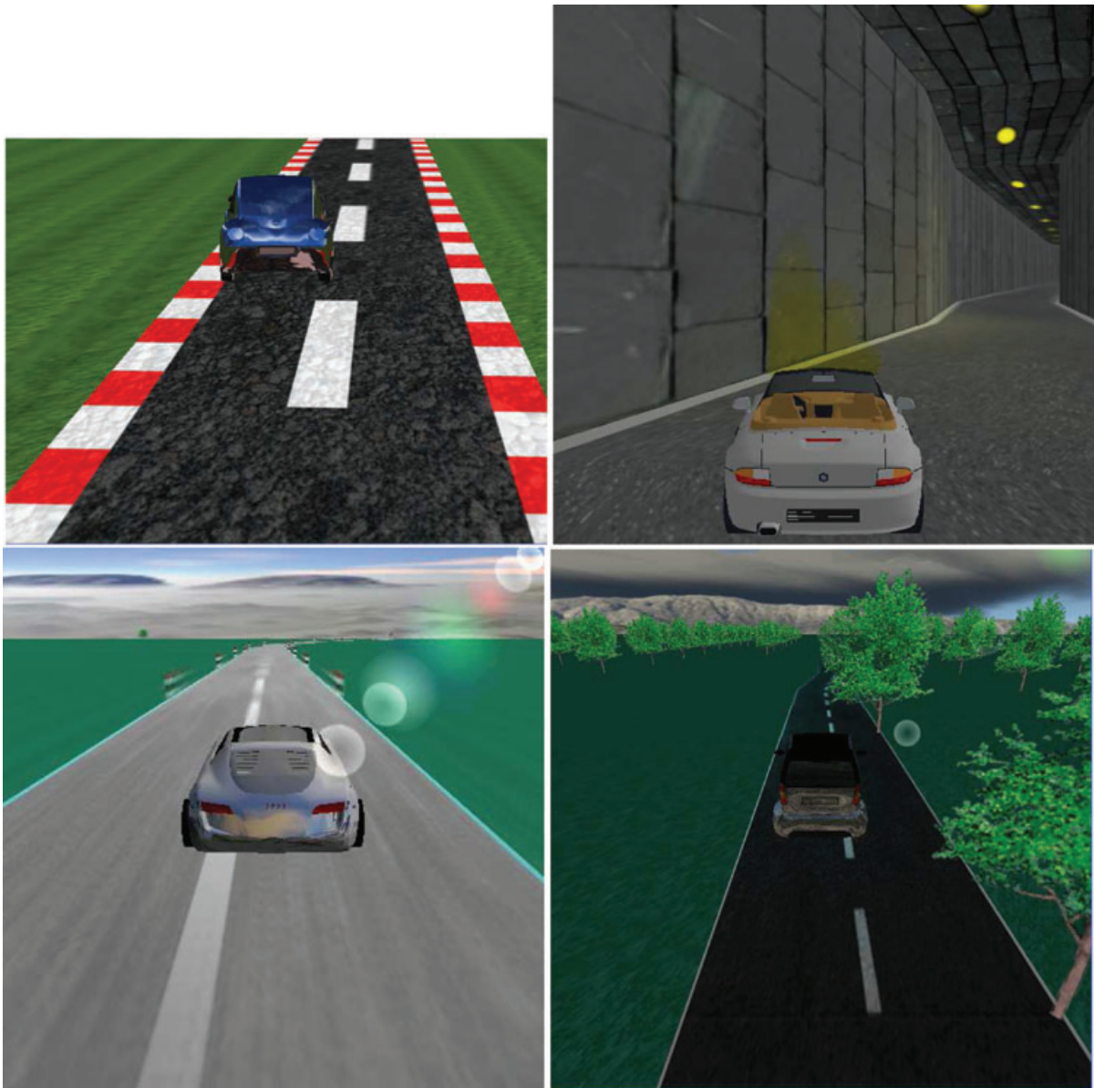
Figure 3: Some clients developed by the students. (Top left-hand panel) Dynamic reflections on the car. (Top right-hand panel) Projective textures for headlights and tunnel lamps faked with textures. (Bottom left-hand panel) Motion blur and lens flare. (Bottom right-hand panel) Billboarding for showing trees.
