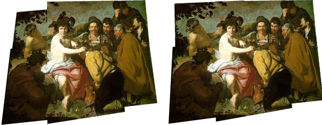
Figure 3. (Left) Circular concatenation of homographies. We can see at the top-left corner the inaccurate registration caused by the accumulation of errors. (Right) Global alignment with incremental approach.
