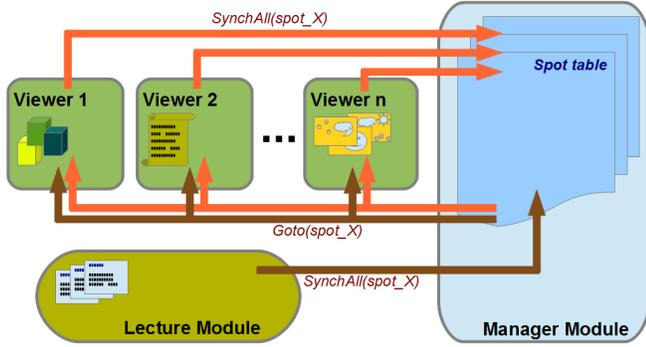
Fig. 1. A scheme of the presentation system: the Manager module communicates with Viewer modules using a synchronization signal. The Manager receives the message and broadcasts a command to focus on the given spot. The Lecture module is able to use the same signals to provide a path through pre-defined spots
