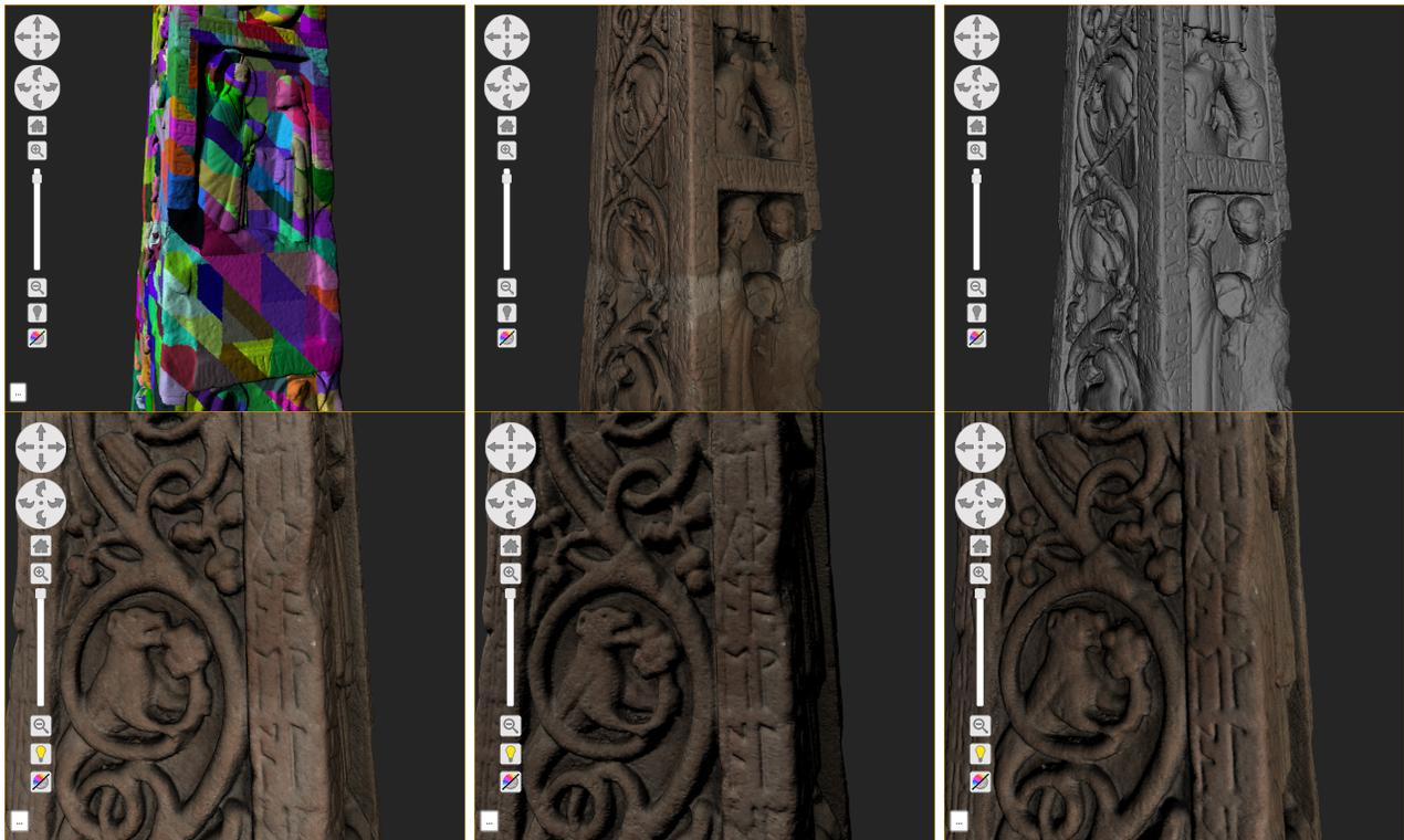
Fig. 3. Screenshots of the rendering of the high-resolution 3D model of the cross. Top left: the patches of the multiresolution rendering engine. Top middle: the geometry with mapped photographic color. Top right: the geometry in a simple Lambertian shading. Bottom row: changing the light direction, to simulate raking light, helps the readability of the carvings.
