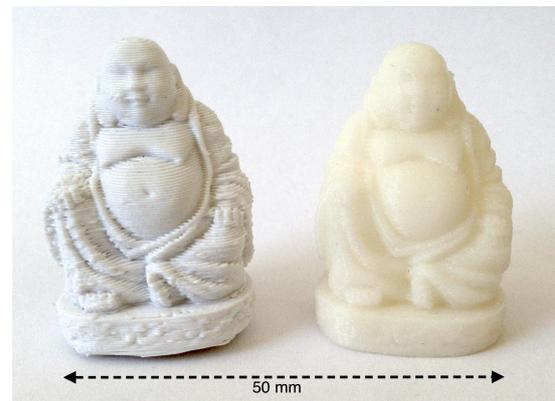
**Figure 3:** Two small buddhas fabricated in ABS using two different FDM machines. Given the limited size of the objects, the layer structure is quite evident. Note that, depending on the appearance properties of the material, the small scale details and the printing artefacts can be evident to a greater or a lesser extent.
