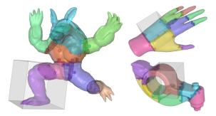
**Figure 16:** The Chopper approach, designed to overcome the working space limitations of current 3D printing technologies.
