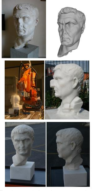
Figure 1: An example of a rapid prototyping project, developed by CNR-ISTI in collaboration with Scienzia Machinale. First row: the original artwork; the digital 3D model obtained using a laser triangulation scanner. Second row: the prototyping machine in action; the reproduction at the end of the automatic reproduction phase. Third row: two images of the final result, after a final manual refinement.
