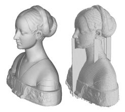
**Figure 4:** Using the FDM approach, printing involves the previous automatic conversion of the 3D model (left) into an approximation composed of the extruded filament (right). This process also includes the creation of vertical columns to support the most protruding parts of the model (such as the chin, nose, ears and hairs of the bust in this figure).
