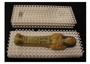
**Figure 10:** An example of a wire-frame lattice structure designed and produced to tightly fit around the shape of the artwork, for packaging and transport.
