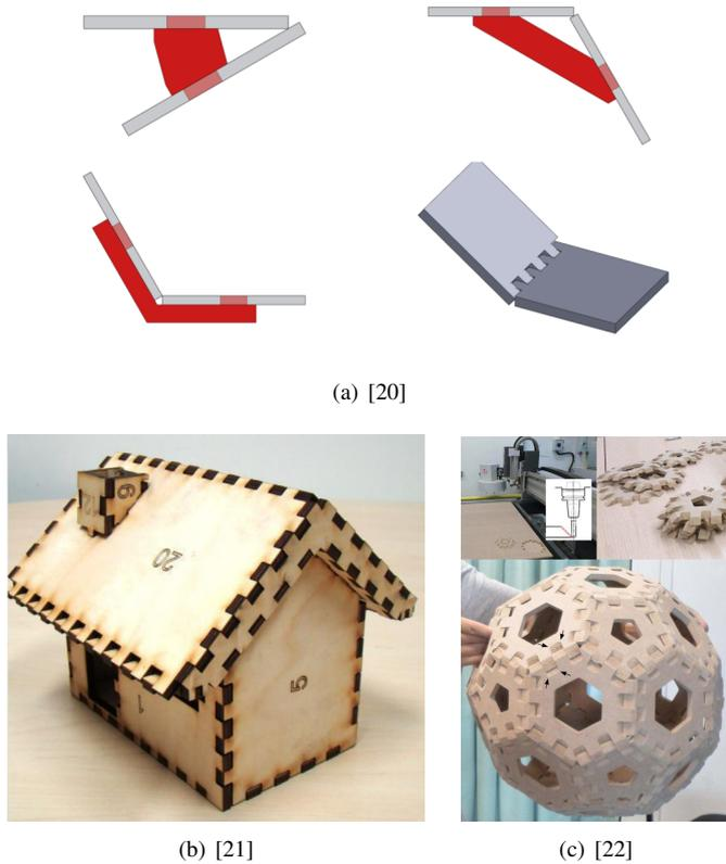
Fig. 4. Joint systems used in related works
