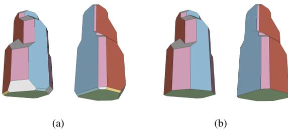
**Fig. 9.** The *Moai* before (a) and after (b) the removal of some facets from its bottom with our user-driven method. The quality of the approximation does not change while the complexity of the model decreases significantly.
