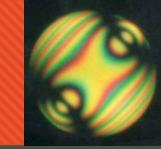
The distance is measured by analyzing the interference between the emitted ray and the returning ray.
