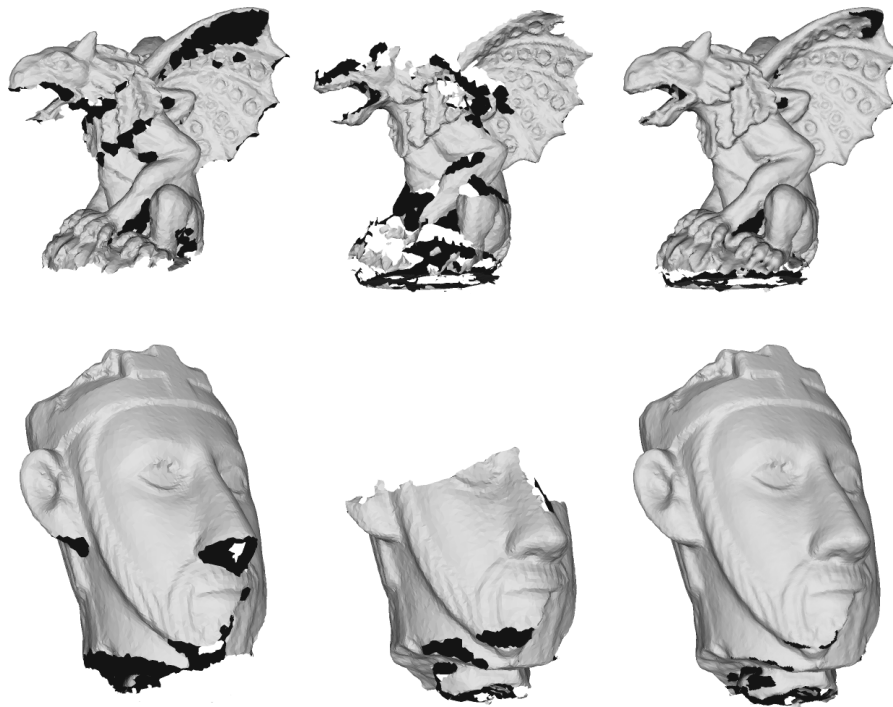
Figure 13. Automatic, unattended scanning of the gargoyle and of the statue head with a rotary table and a mirror; columns from left to right: the upper part acquired directly by the scanner, the lower part, acquired through reflection and the merged meshes.
