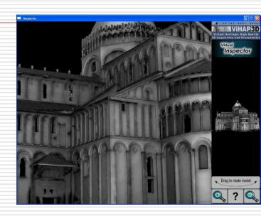
The distance of sampled point is obtained by measuring the time between the laser impulse and the sensor read-back, divided by (two times) the speed of light...
