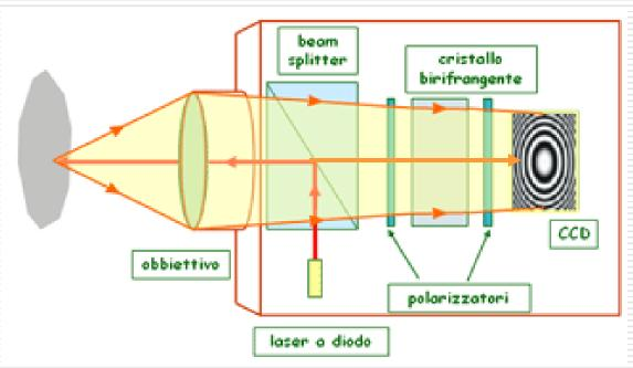
The direct and the reflected beam arrive on the crystal, frequencies are no longer aligned, producing interference... interference bands are used to determine the distance of the sample
