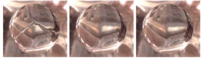
Figure 7: Continuity handling comparison. Left and Center : isolated surface algorithm (section 5.2) without and with dynamic gutter. In the center picture, small discontinuities might still be spotted. Right : algorithm designed for seamless continuity (section 5.3).
