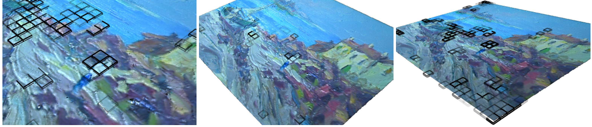
Figure 5: Behaviour of our view dependent adaptive scheme. For close-ups (left) or at grazing angles (right), more boxes are automatically selected to be rendered with relief mapping so as to prevent parallax error where relief becomes significant.
