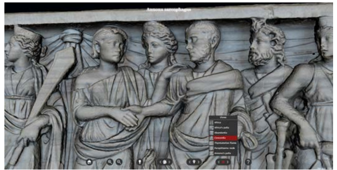
Fig. 6. 3DHOP supports the definition and visualization of a predefined set of views, selected to show the most representative polychrome areas on the Annona sarcophagus.
