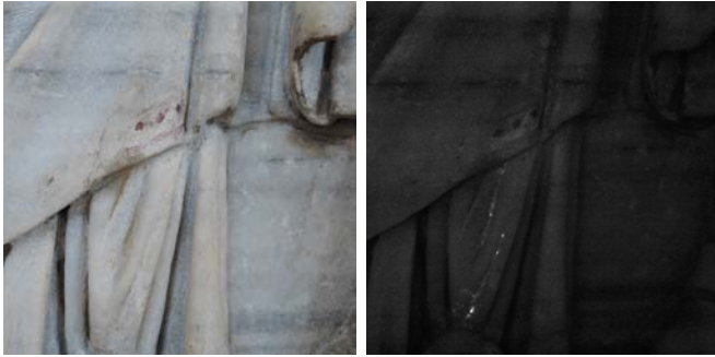
Fig. 12. Polychrome detail of the ornamental edge of the Annona's palla (left) and the same area in VIL imaging that shows the distribution of glowing white particles of Egyptian blue (right). On the white band the EB is located as scattered particles, while on the stola a compact layer is observed.
