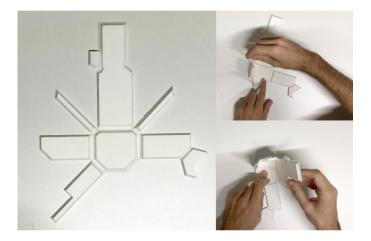
Fig. 18. An example of the assembly process for the Moai model.
