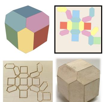
Fig. 22. Manufacturing of a modified sphere. From top left to bottom right: the digital simplified model, its unfolding, the carved sheet of plywood, and a picture of the fabricated model.
