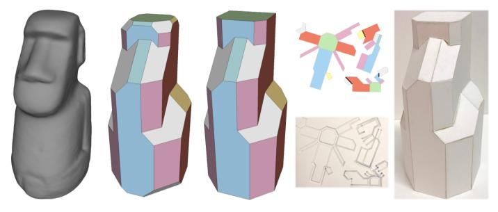
Fig. 1. From left to right: the input digital model; the result of the automatic simplification step (Section 3); the clean model after spurious facets removal (Section 4); on top the unfolding plan for fabrication and on bottom the corresponding carved sheet (Section 5); the final assembled model manufactured using a CNC milling machine and manually folded and glued (Section 6).
