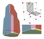
Fig. 7. Dihedral angles of 90° cannot be obtained using the Marching Cubes algorithm. There will always be small facets as junctions between orthogonal facets. In most of cases, these facets are not suitable for the proposed fabrication task and they could not contribute for a better approximation.
